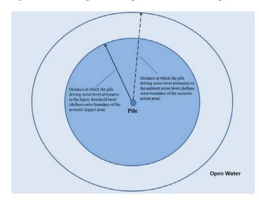
Figure 3.2 Pile driving acoustic impact and action area in open water.
